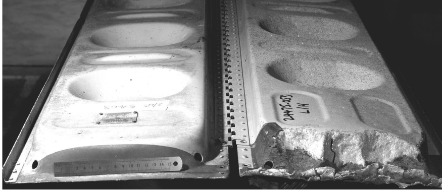
Fig. 1 Photograph of C-130 Hercules main gear undercarriage bay doors. The undamaged trailing edge of the door is shown on the left and the impact damaged leading edge of the component is shown on the right.
